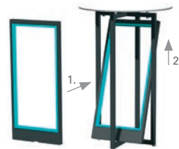
folding-system of the SET Table
