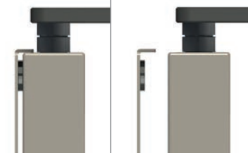
mounting by magnets and small hooks
